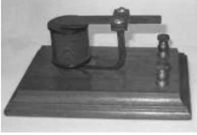
Fig. 1.2. Receiver of Alexander Graham Bell's "harmonic telegraph" which used reeds responsive to different frequencies. Photo of replica of original equipment used with permission of Telecommunications Museum, LaSalle, Quebec, Canada.
